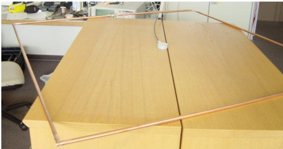
Figure 8: Entire antenna construction
