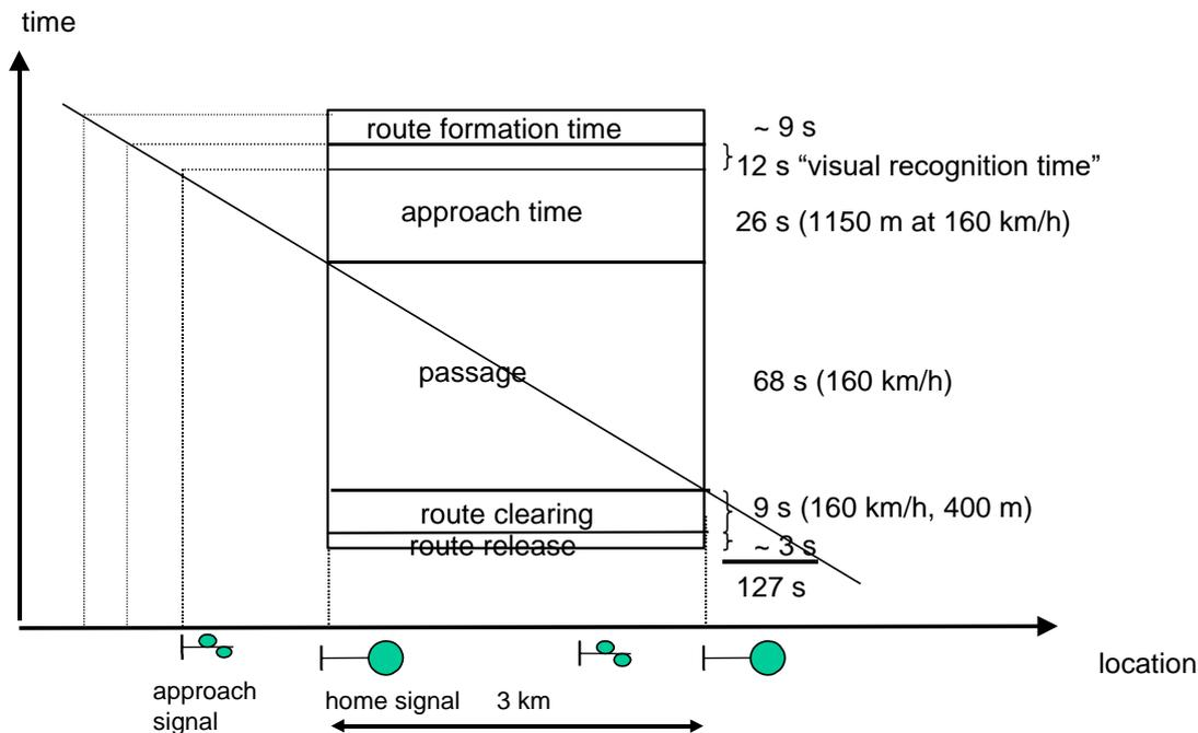
In case of an intermittent, signal based train control system, the “visual recognition time” requires that the trackside elements are set and the signal shows “green” 12 s before the train passes the approach signal to keep traffic fluent, because otherwise the driver would start to apply the service brake to stop the train as soon as he recognizes the approach signal indicating to stop ahead.
