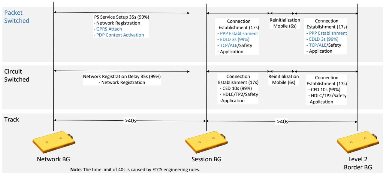
**Figure 2: Relationship between trackside elements and QoS parameters**
