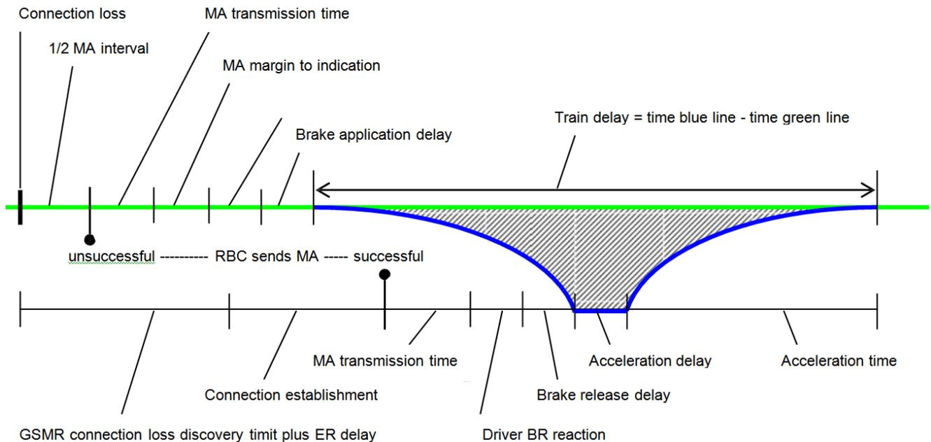
Figure 19: Loss of Connection
