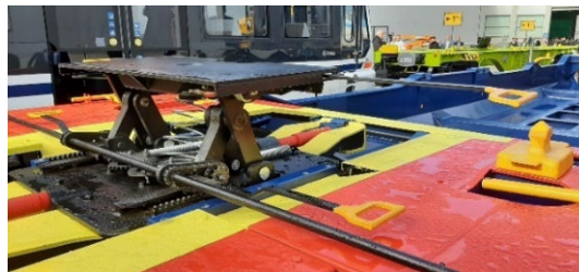
Figure 4 – Example of device to secure semi-trailer (from Innotrans 2024)
