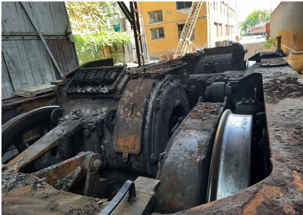
Fig. 4.14. Condition of the bogie and the traction motor after the fire
