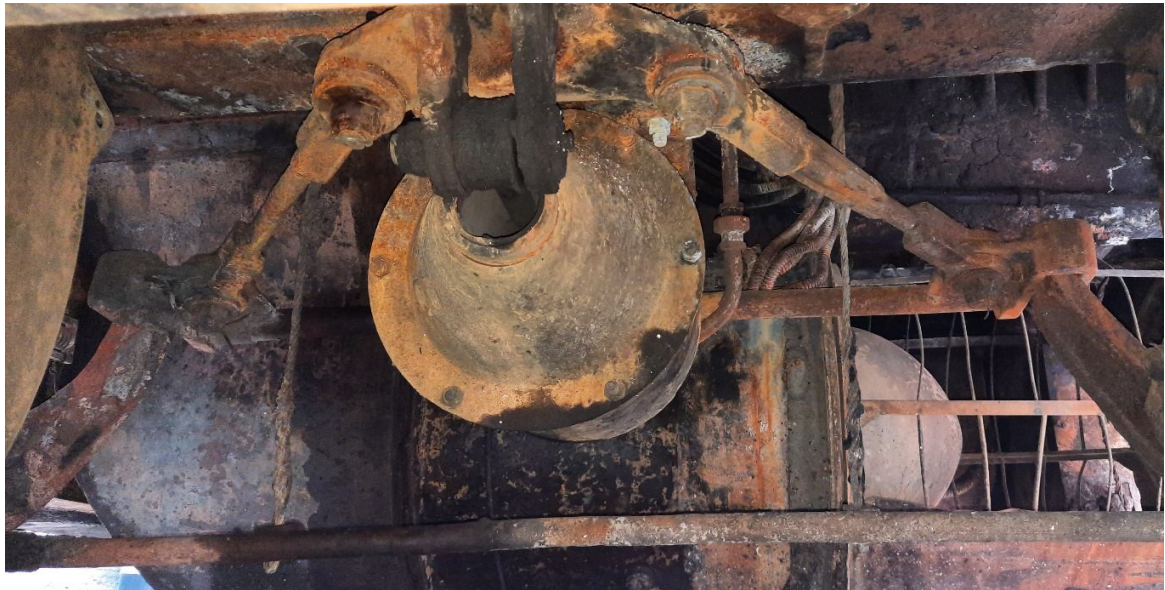
Fig. 4.13. Condition of the elements under the locomotive frame after the fire
