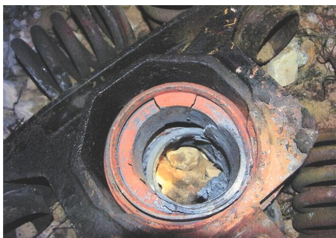
Figure 9 No. 1 wheel axlebox with the remains of the failed cartridge bearing (external side)
