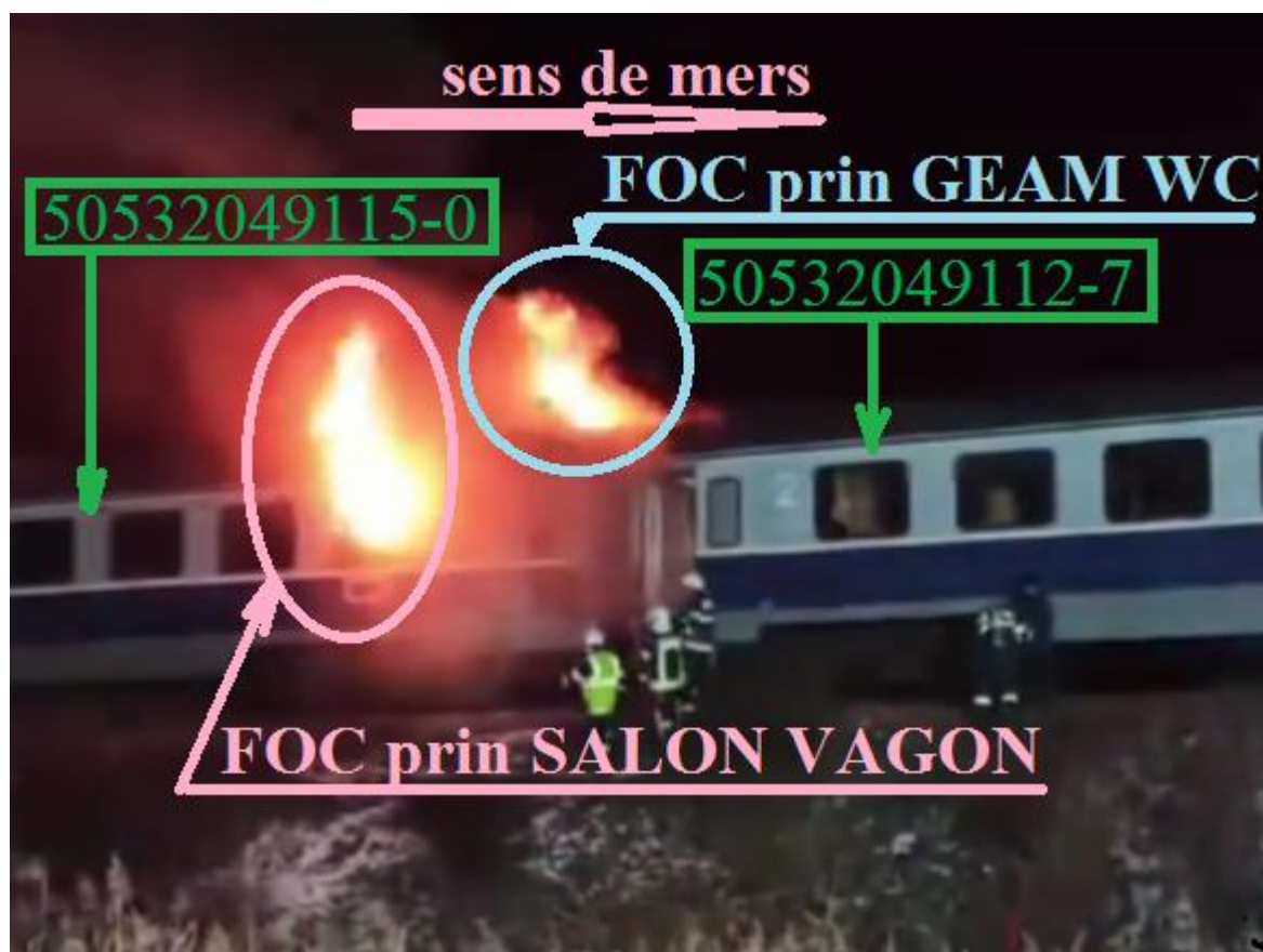
Image no.16 - Fire between the 2nd and 3rd wagon of the train
