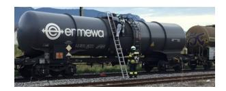
In both cases, the leaking hydrochloric acid posed serious risks, but quick action prevented further harm. The leaks were attributed to failures in the internal protective lining of the wagons, which had not been detected during mandatory inspections by various testing centers.
