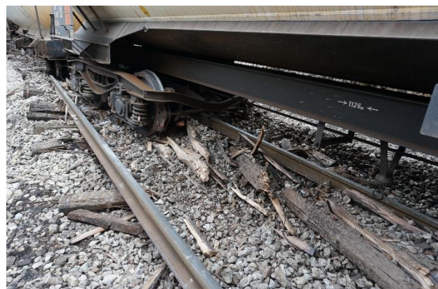
Figure 3.4.4.2: Appearance of the parts of derailed wagons
