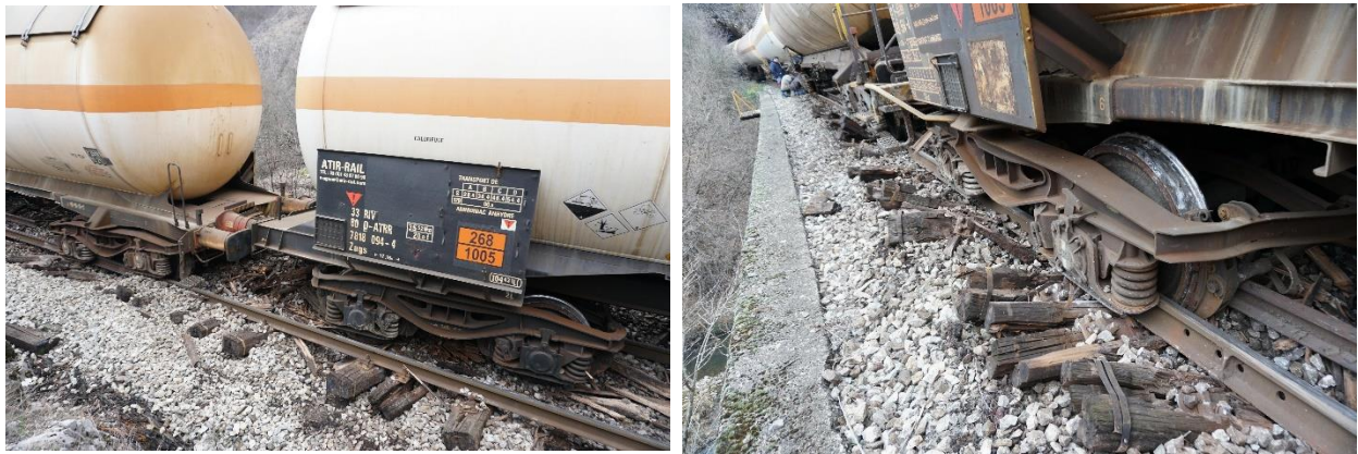
Figure 3.4.4.3: Appearance of the parts of derailed wagons
