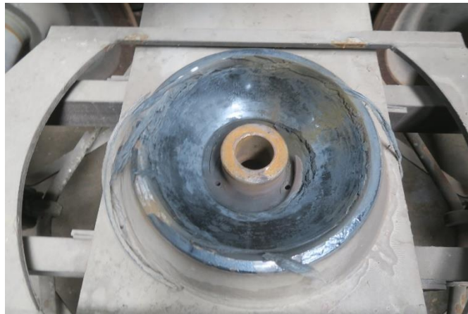
Figure 4.2.6.1: The condition of the lower center bowl on wagon No. 33 87 7814 136-0 at housings 7 and 8
