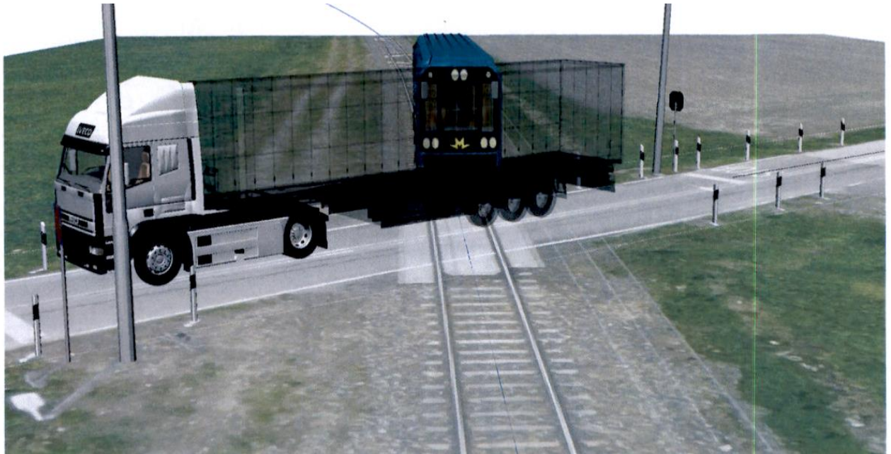
Figure 3 – Relative positions of vehicles at the time of their collision (source: Opinion of a forensic expert)
