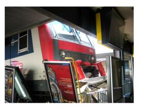
On Monday 13 August 2007 at 10:27 a.m., Transilien train No. 141 280 running between Paris-Invalides and Versailles Rive Gauche collided with the buffers of track 3 in the Versailles Rive Gauche station at a speed of 6 kph.
