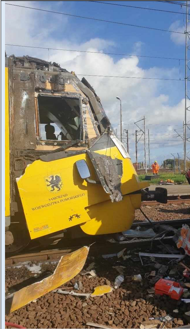
Photograph 30 - Consequences of the occurrence - damage to SA138-004 (source: own material of PKBWK)
