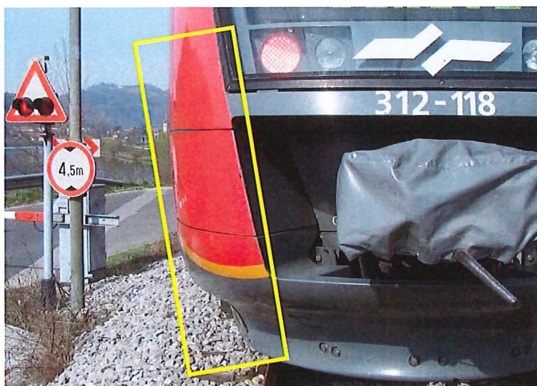
Image 1: The yellow square shows the marks and minor damage to the sheet metal
