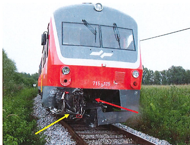
Image 3: The red arrow shows the completely destroyed automated coupler of train No. 3375 and the yellow arrow shows the front right side of the control unit of DMU 715-125.
