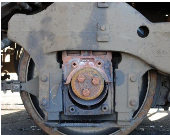
Figure 5 – Failed bearing on locomotive 233
