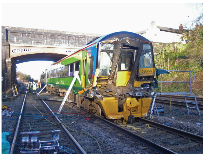
Figure 1: View of the train following collision with the footbridge, Barrow on Soar Report 18/2008.
