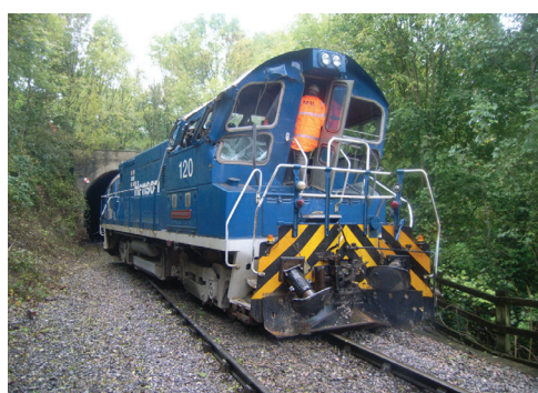
Collision damage to derailed locomotive
