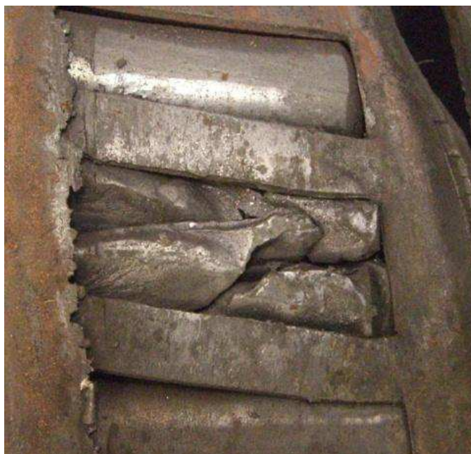
Figure 10: Fractured Outboard Roller 11
