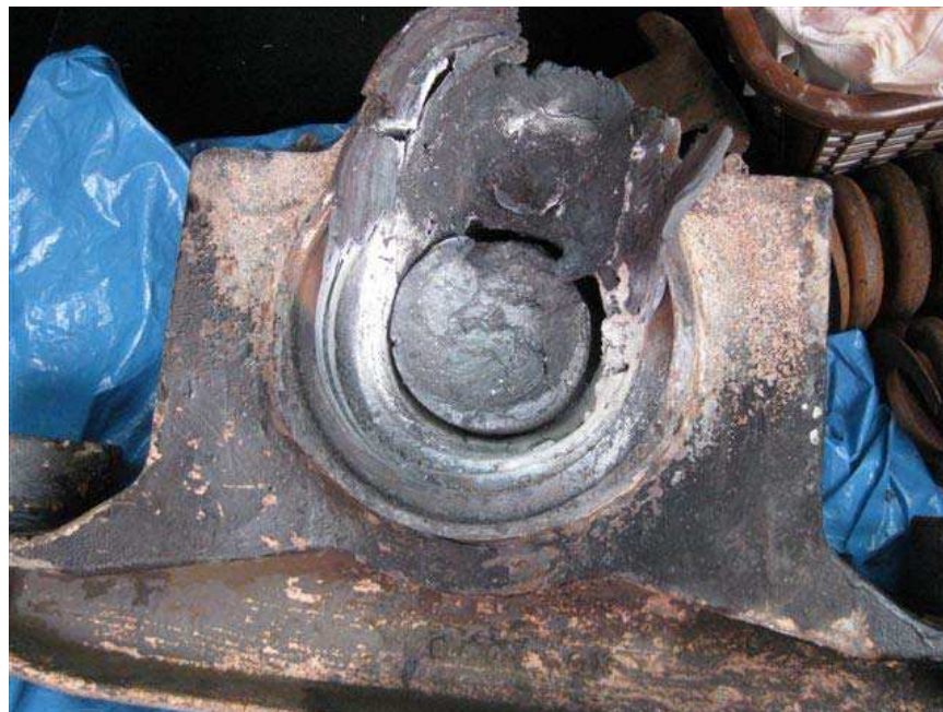
Figure 3: Example of a Bearing Failure 6
