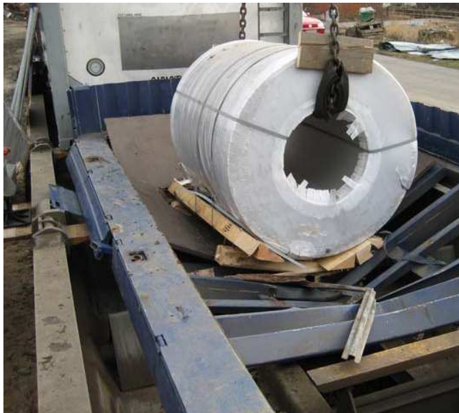
Figure 11: Inappropriate Train Loading 12
