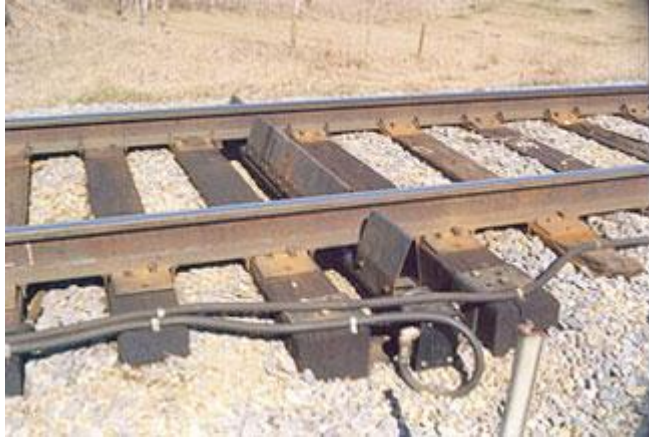
Figure 5: Typical US derailment and dragging object detector
