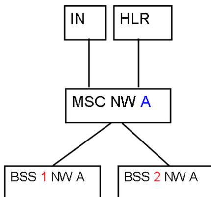
Figure 4.5: Test scenario III - focus to EIRENE networks with different BSS
