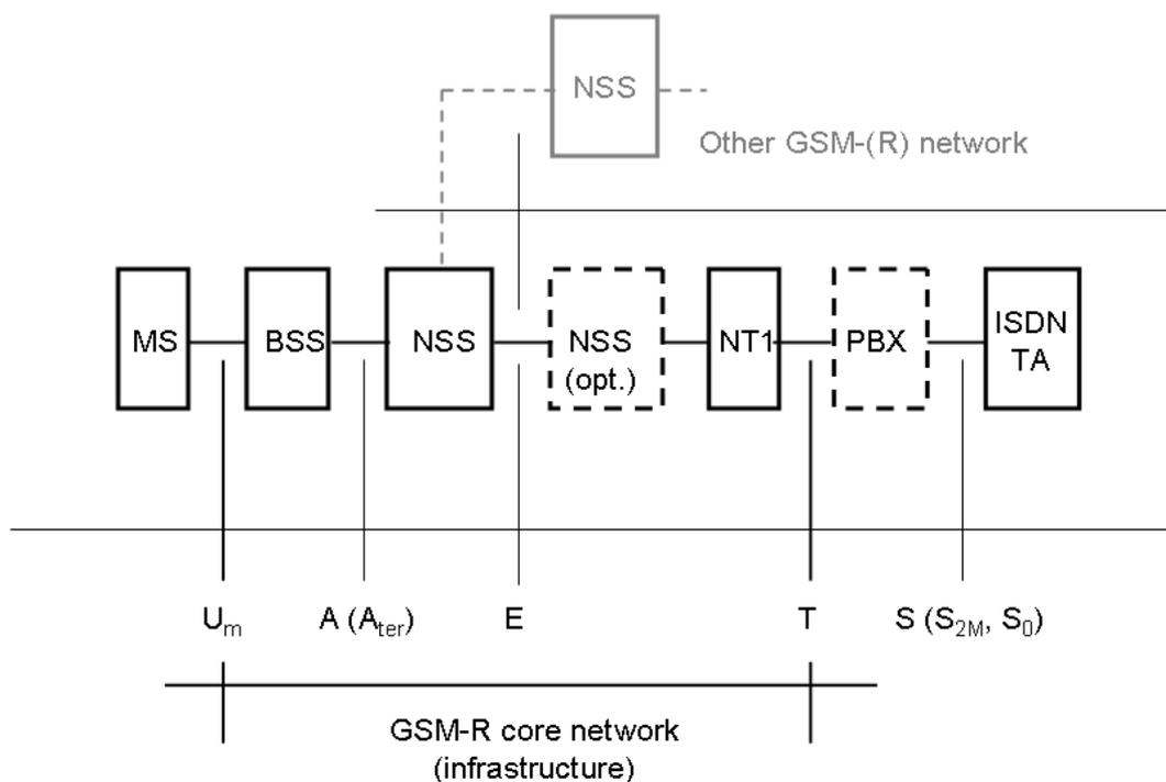
Figure 4.1: Reference configuration and the interfaces of an EIRENE network
