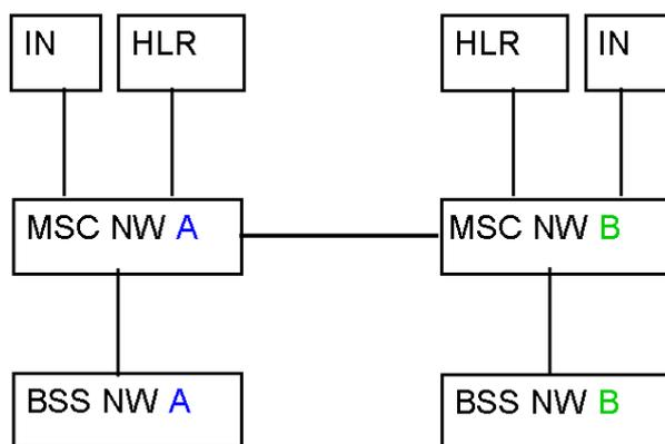
Figure 4.3: Test scenario I - Interconnection of two EIRENE networks
