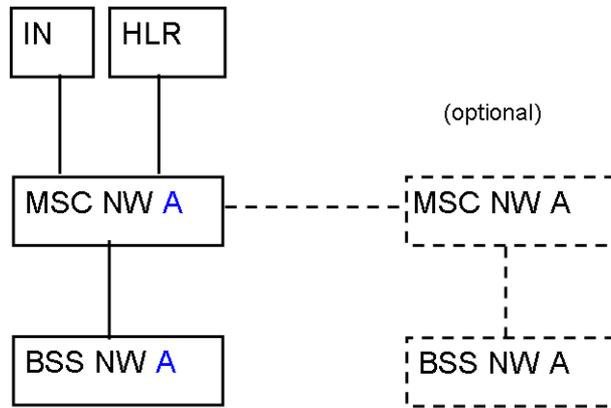
Figure 4.4: Test scenario II - configuration of a single EIRENE networks
