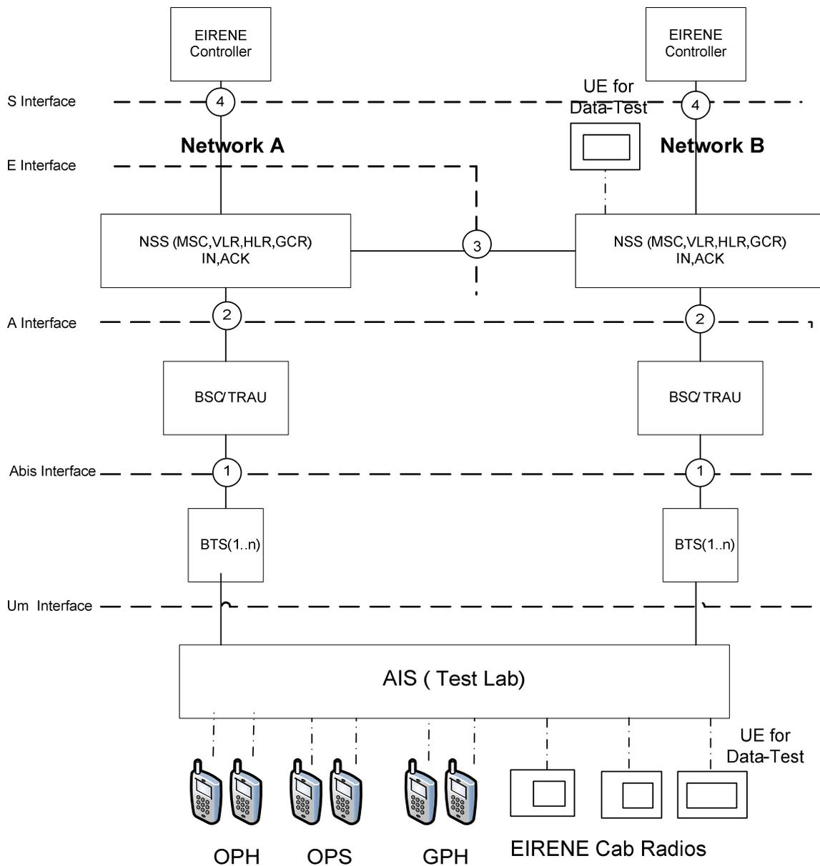
Figure 4.7: Generic IOT test configuration for GSM-R networks
