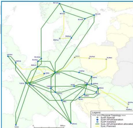
European GSM-R networks are interconnected via two hubs (and not via point-to-point connections)
