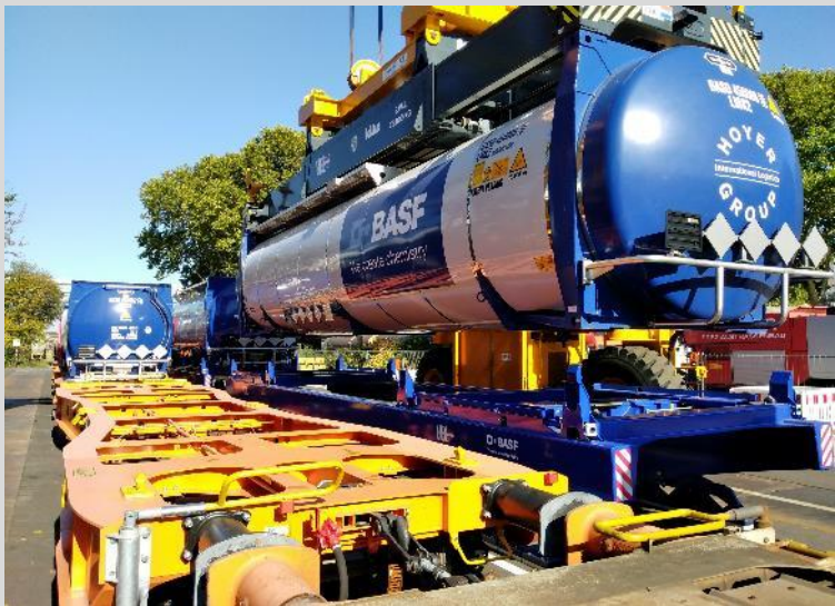
BASF Class Tank Containers up to 73,000 Liter volume 66 tons payload
