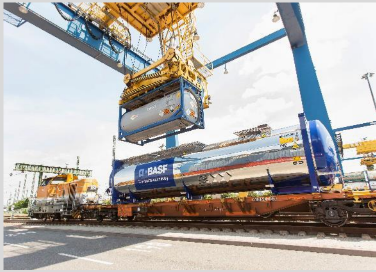
Standard tank container 25,000 – 36,000 Liter volume 25 tons payload
