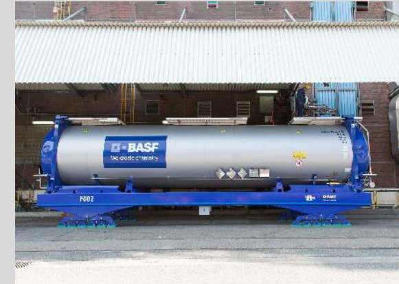
Frame makes loading without AGV possible
