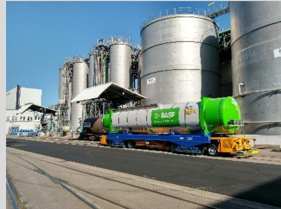
Autonomous onsite AGV transport
