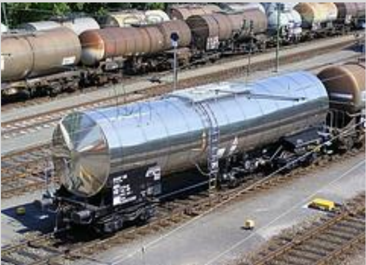
Classical rail tank car 70,000 Liter volume 64 tons payload
