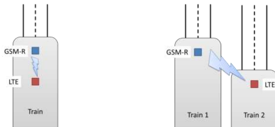
Figure 5-29: Critical scenarios for interference from GSM-R MS to LTE UE
