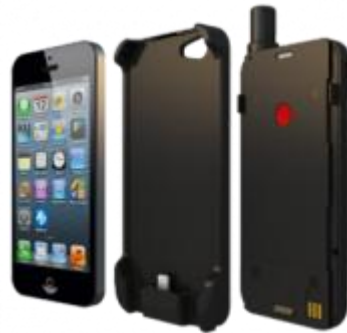
Figure 26: Thuraya SatSleeve terminals (enable regular GSM terminals as a Satcom terminals)
