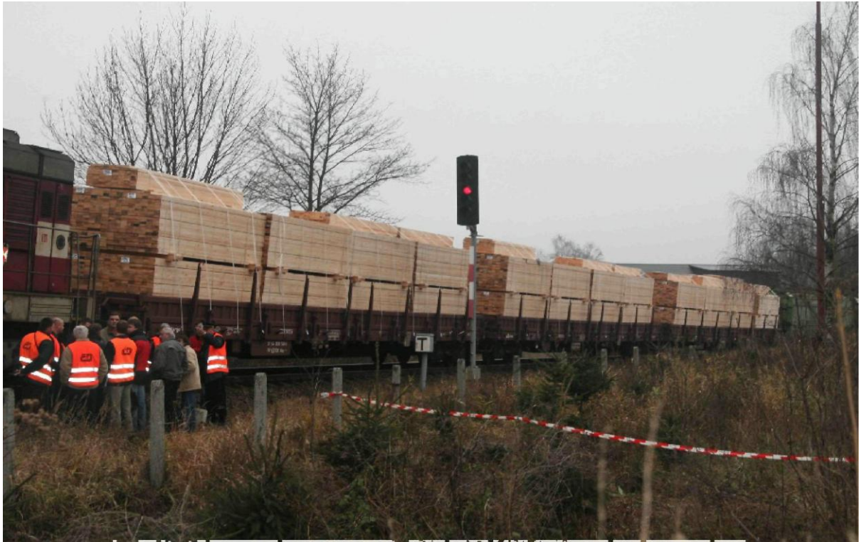
Appendix 5: Position of the shunting freight train in relation to the "S" entry signalling device
