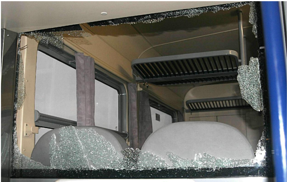
Appendix 6: Broken glazed partition
