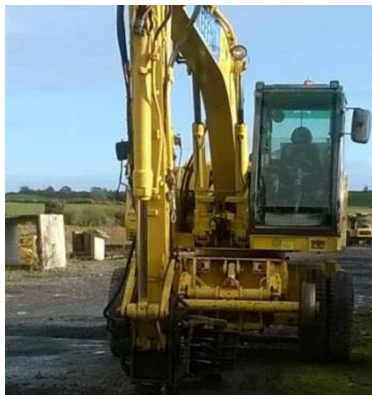
Figure 10 – RRV with rail grab attachment
