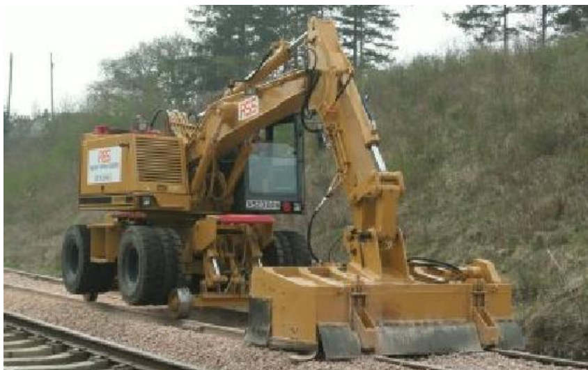
Figure 43 – RRV with brushbox (similar to RRV involved in accident)
