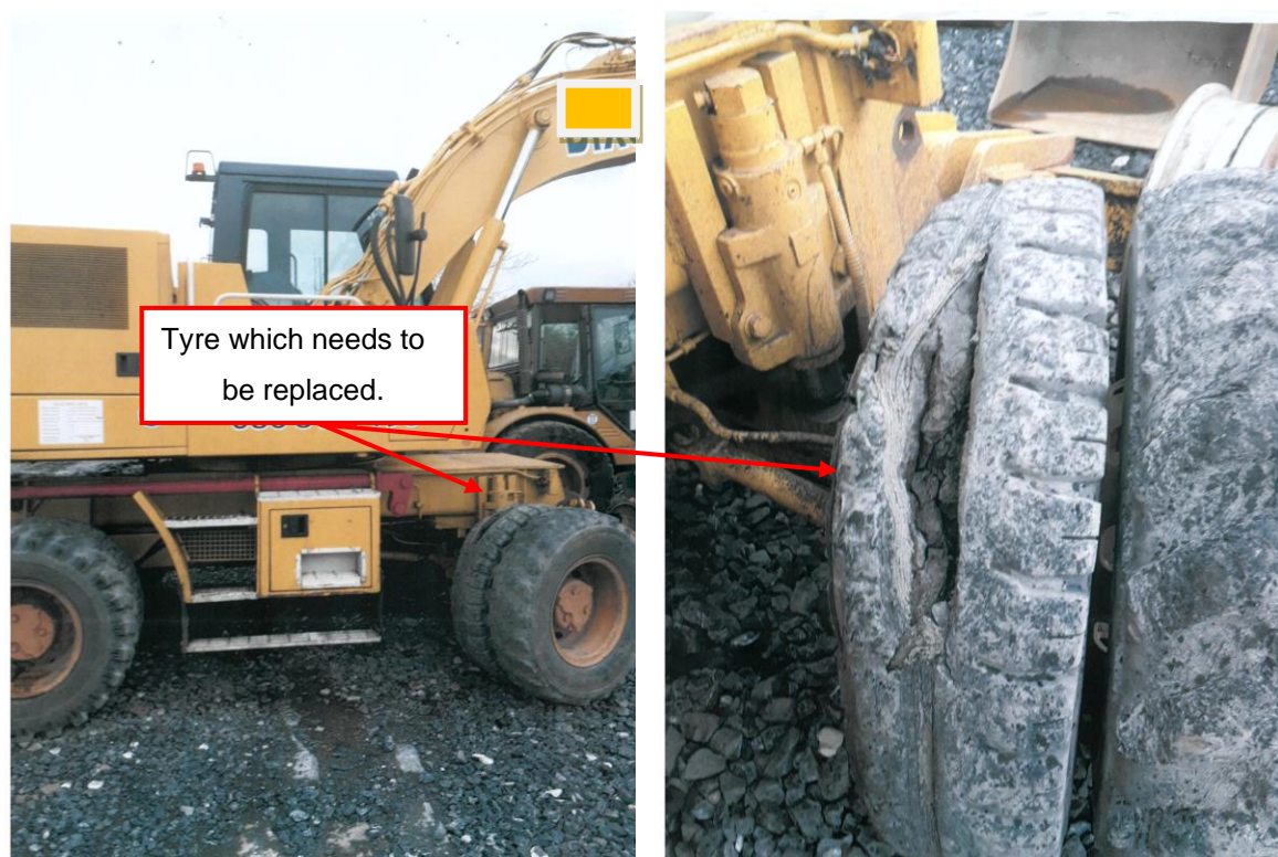
Figure 7 – Tyre identified by IÉ-IM which needs replacement
