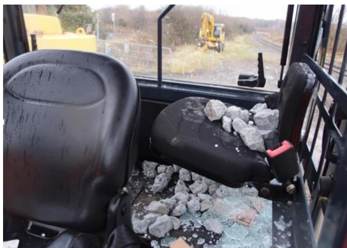
Figure 18 – Damage to RRV
