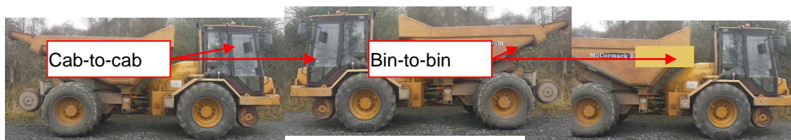
Figure 15 – Cab-to-cab / bin-to-bin orientation
