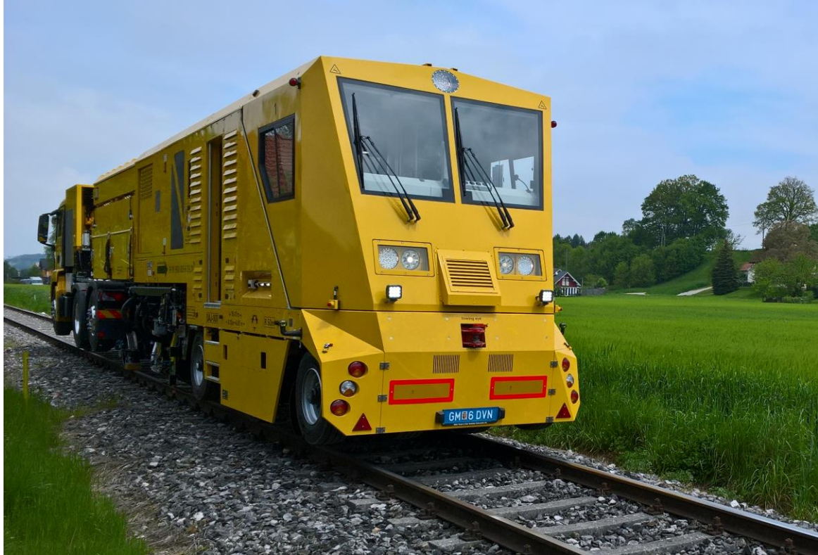
Figure 4 – New Type 9A RRV on IÉ network
