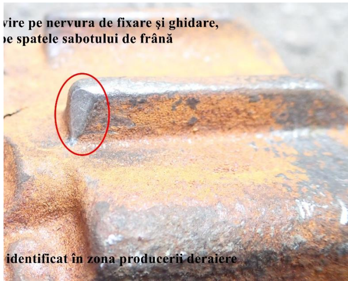
Picture no.2 – mark of hit on the pin for fastening and guiding of the brake shoe identified at the derailment site
