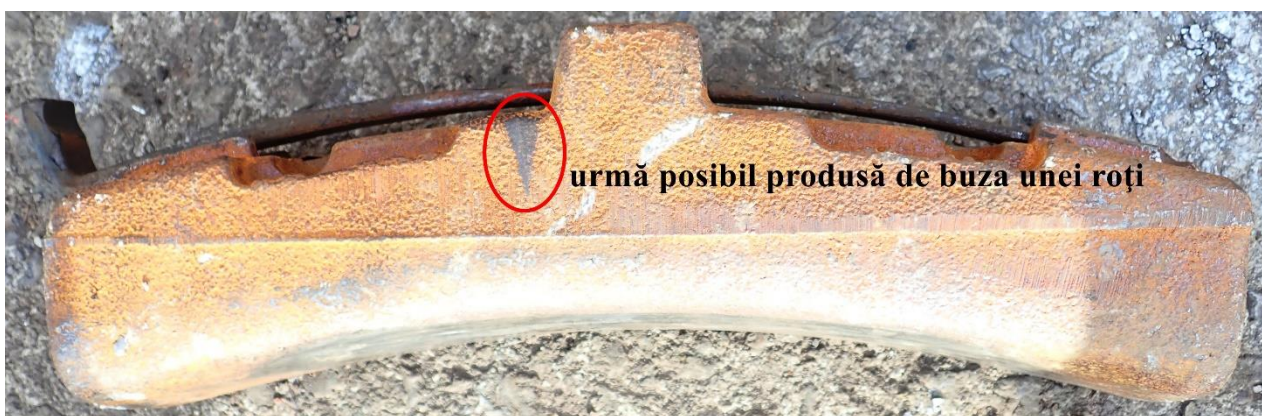
Picture no.1 – the brake shoe found at the first derailment mark
