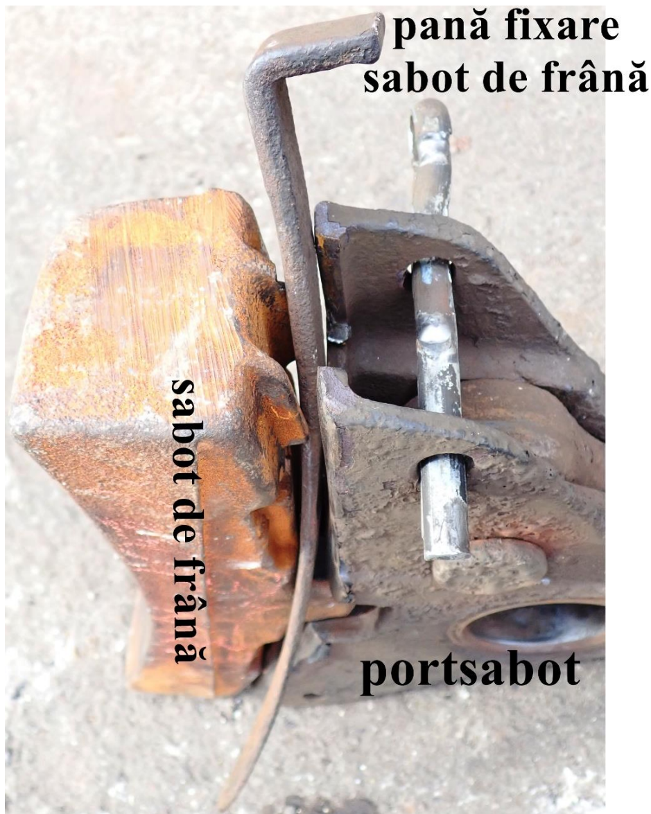
Picture no.4 – ensemble brake shoe – brake shoe holder having the key put between those two elements
