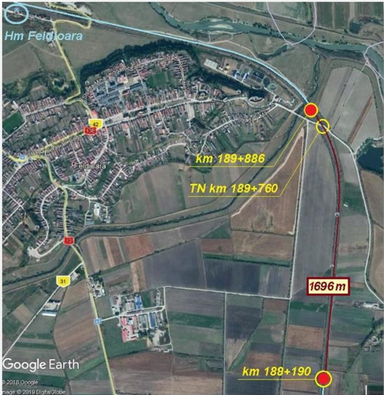
Figure no.3 – accident site – satellite capture. The distance of 1696 m ran by the wagon with the bogie no.2 derailed
