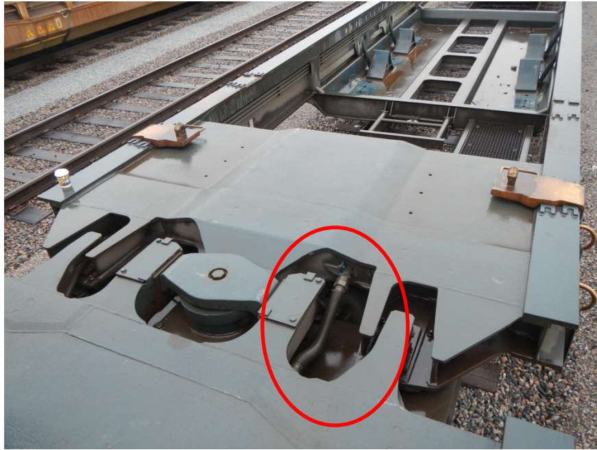
Figure 4. The red circle in the picture shows the hose in question over the middle bogie.
