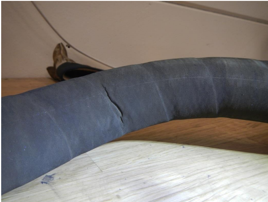
Figure 5. The examined hose material has a crease on the surface.
