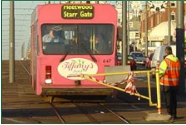
Figure 3: Southbound tram approaching the temporary swinging gate at Gynn Square
