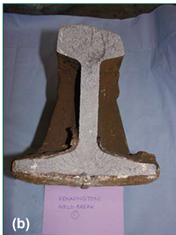
Figure 6: Broken left-hand rail from Urchfont
