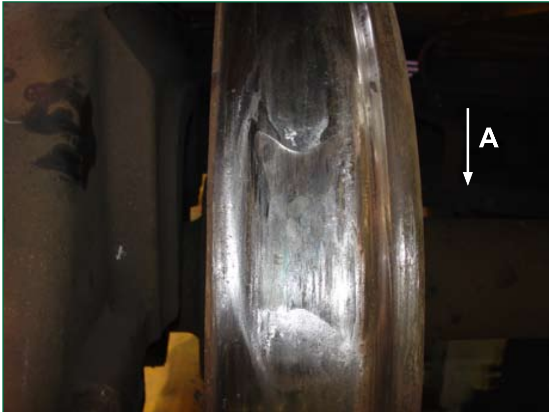
Figure 5: Flat on wheel 3 of axle 3 (serial no. ZB 362/9/057) on wagon NLU 29553
