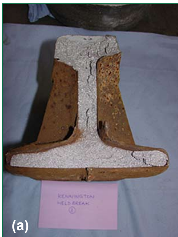
Figure 7: Broken left (a) and right (b) rails from Kennington
