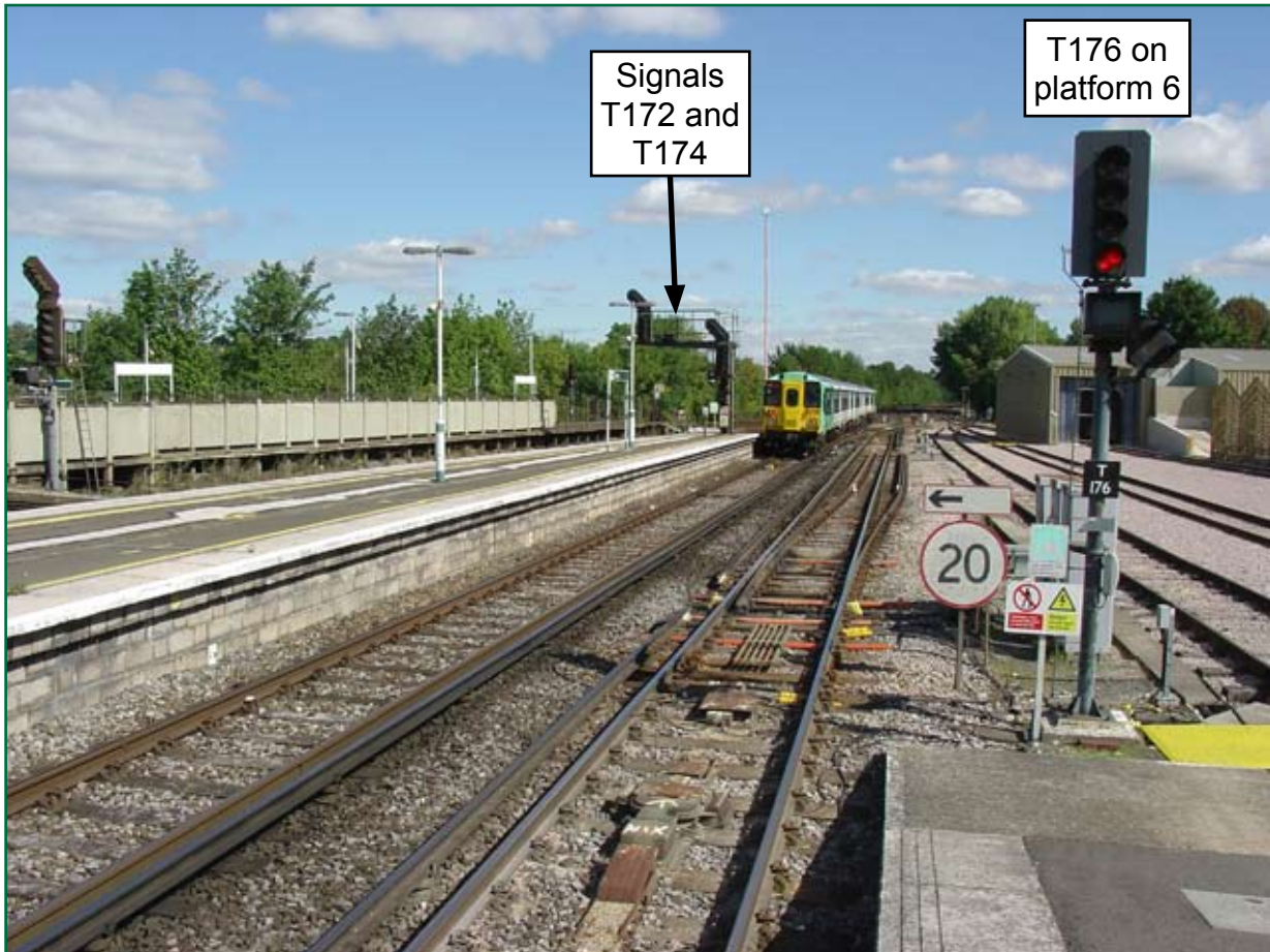
Figure 9: Signal T176 at the London end of platform 6 at Purley showing similarity to T174 on platform 5
