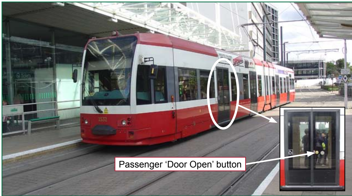
Figure 3: Croydon tram, showing doors and push button (inset)
