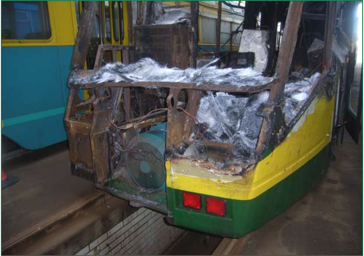
Figure 4: Fire damage to the exterior at the B end
