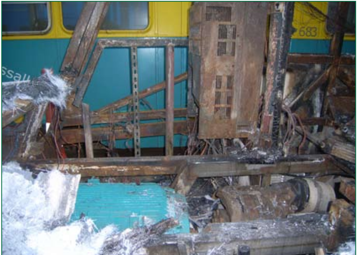
Figure 5: Fire damage to the B end driving position
