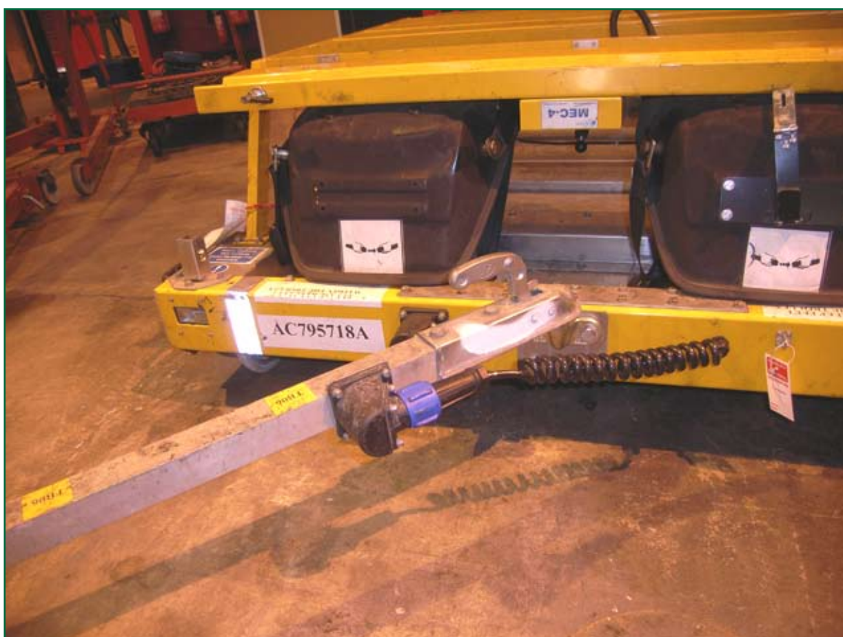
Figure 5: Tow bar and electrical connection
