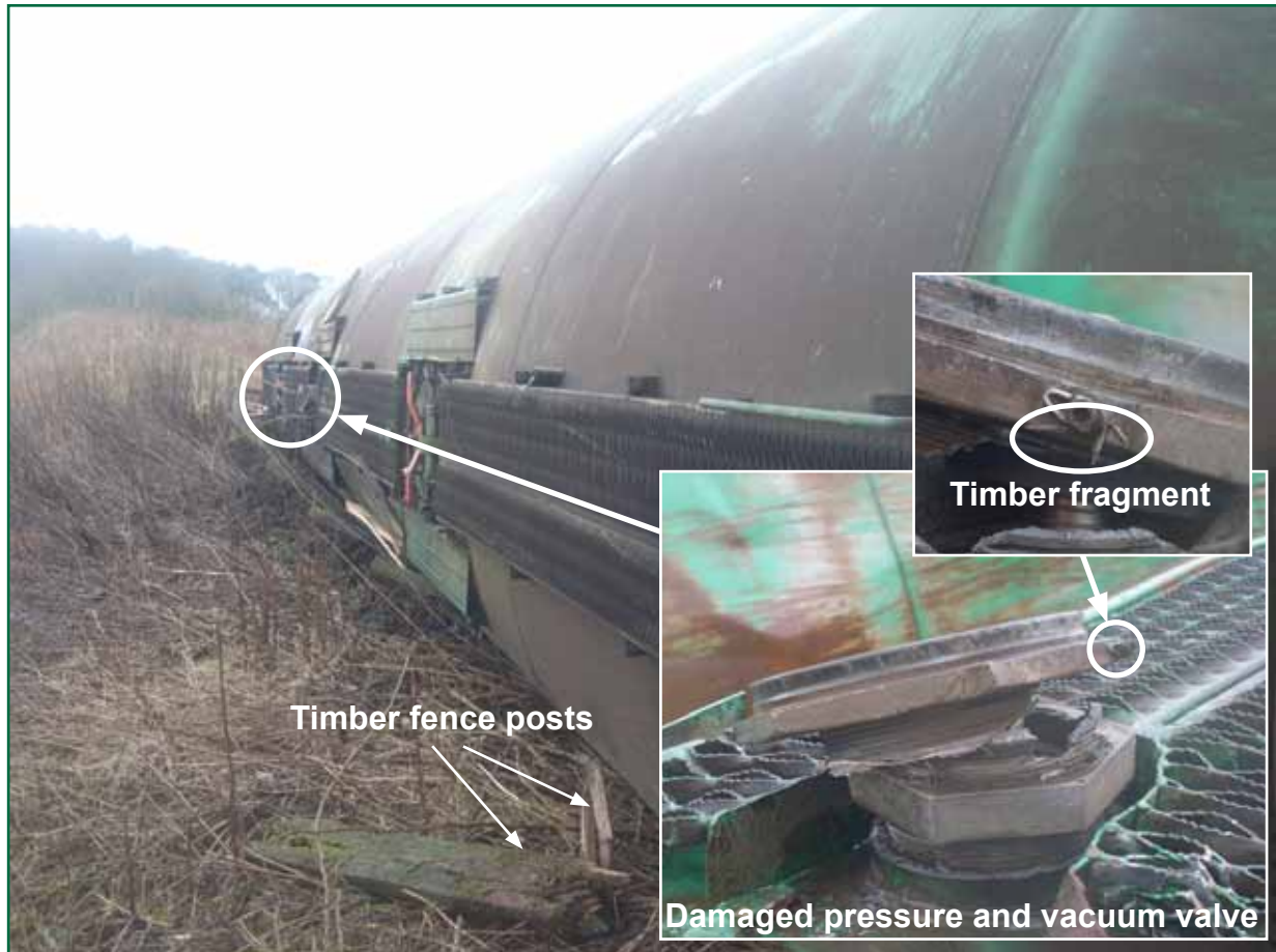
Figure 24: Damaged pressure and vacuum valve on wagon 7
