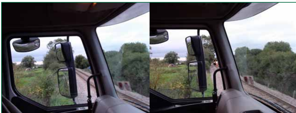
Figure 10: Effect on tanker driver's view of an approaching train caused by the mirror cluster on near-side of tanker (Photographs from the sighting tests on 3 October 2010)
