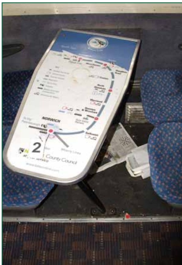
Figure 13: Typical example of table deformation
