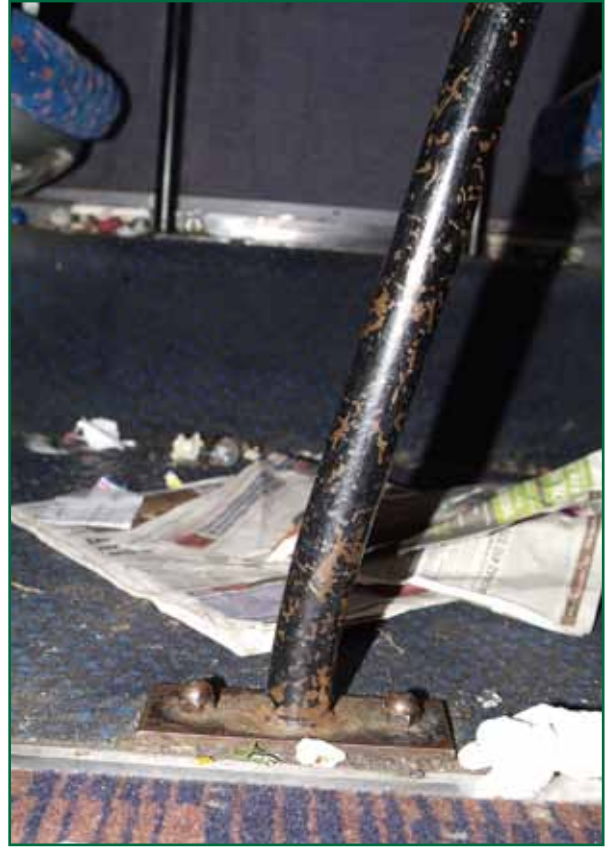
Figures 15 and 16: Damaged legs at base of interior tables within the vehicles
