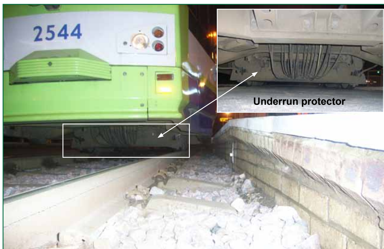
Figure 7: Front of tram showing underrun protector
