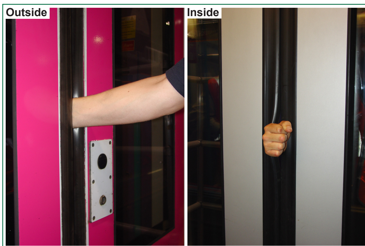
Figure 10: Adult male wrist (approximately 45 mm by 70 mm) trapped in a door detected as closed and locked
