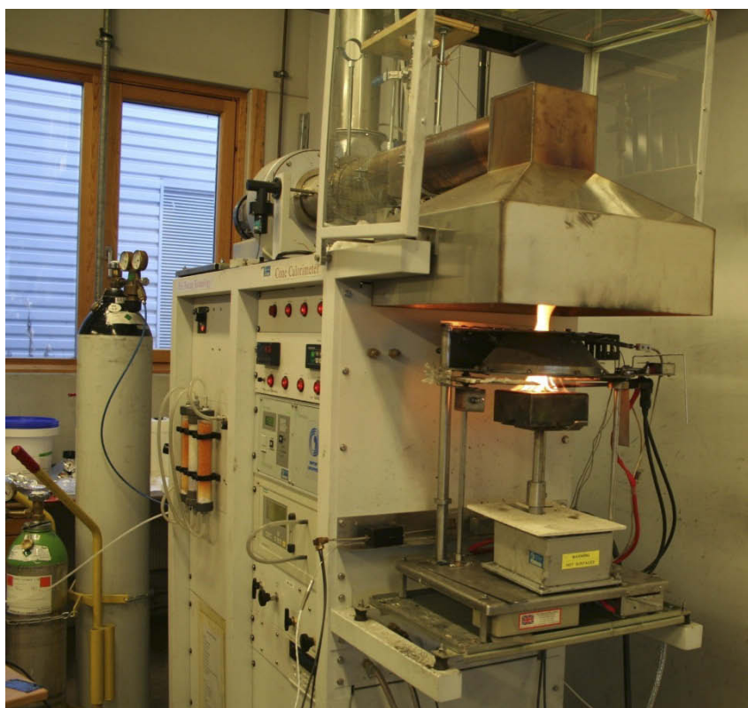
Figur 4-2 Konkalorimeter under test
