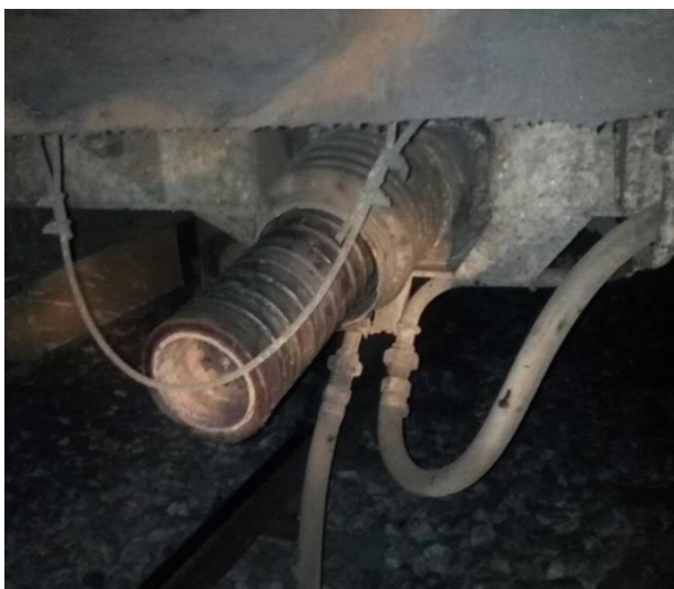
Figure 3.4.4.1: Appearance of a part of the decoupled coupling on the trailer 416-004
