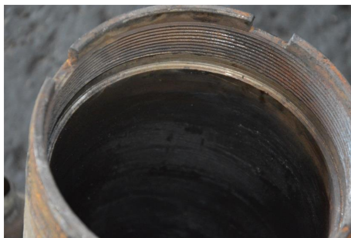
Figure 4.2.3.2: Thread of the housing of the coupling's spring from trailer 416-004
