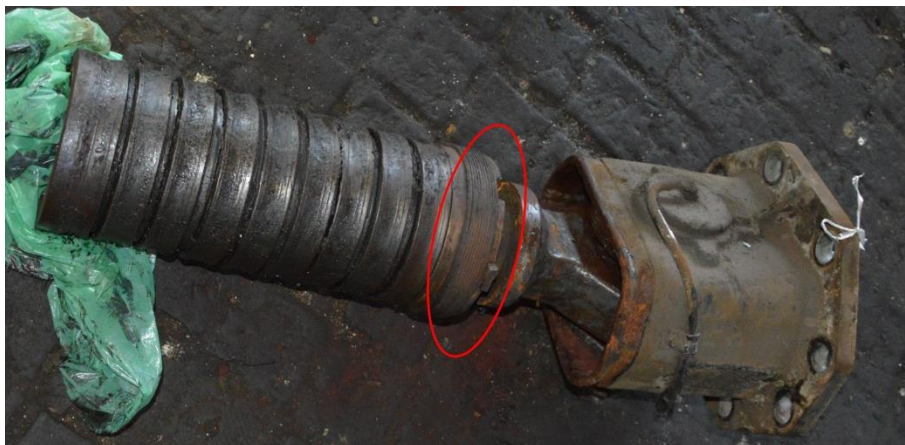
Figure 4.2.3.1: Pulled out set of the draw bar (the thread part is encircled) demounted from the trailer 416-004
