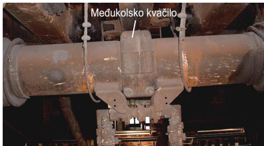
Picture 2.2.2.2: Appearance of the coupling between vehicles installed in EMV series 412/416
