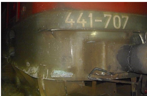
Fig 3.4.4.1: Review of the damage on EMV 441-707
