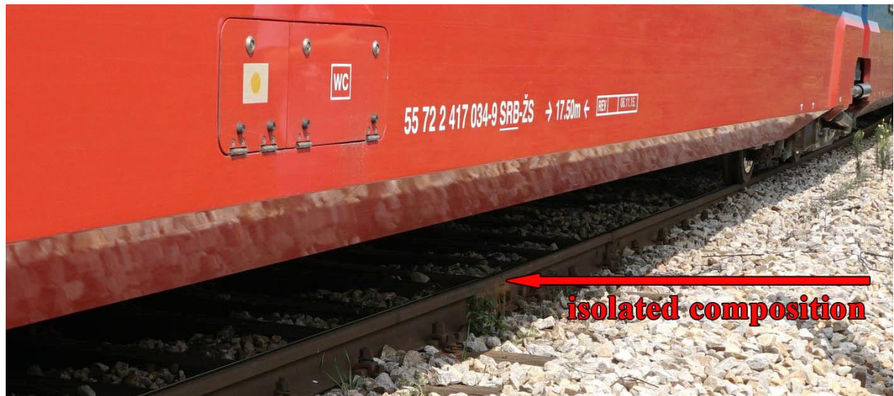
Figure 4.1.6: Position of the isolated composition between the automatic block sections IpE3 and IpE4 relative to the EMV 413/417-033/034
