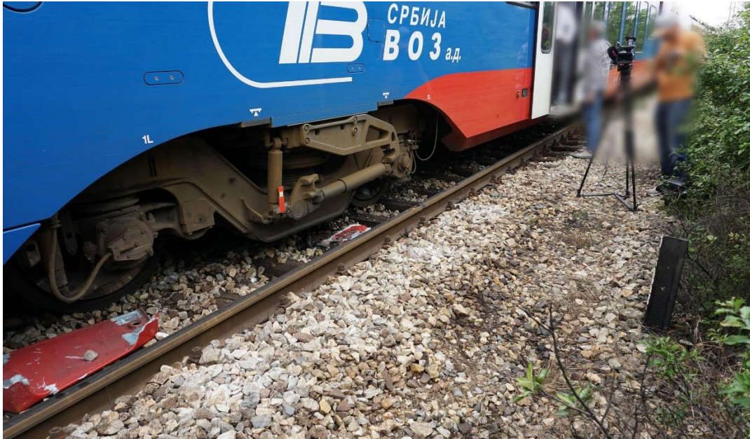
Figure 4.1.4: Appearance of the derailed bogie EMV 413/417-033/034
