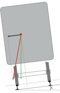
In the Froidmont tunnel, the curved track was laid with a cant (h) calculated for a design velocity of 90 km/h.
