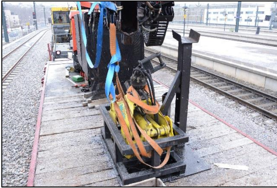
Figur 4: Holdebrakett for transportsikring. Foto: SHT
