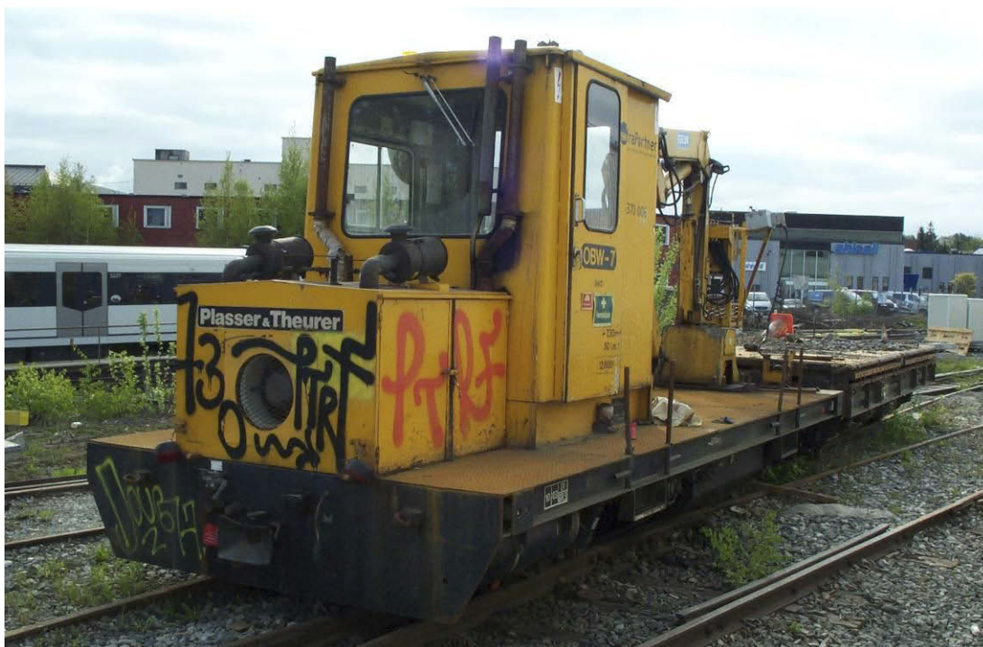
Figur 2: Plasser & Theurer OBW 7 dieseldrevet skinnetraktor (kilde: KTP AS v/ Trygve Pedersen).
