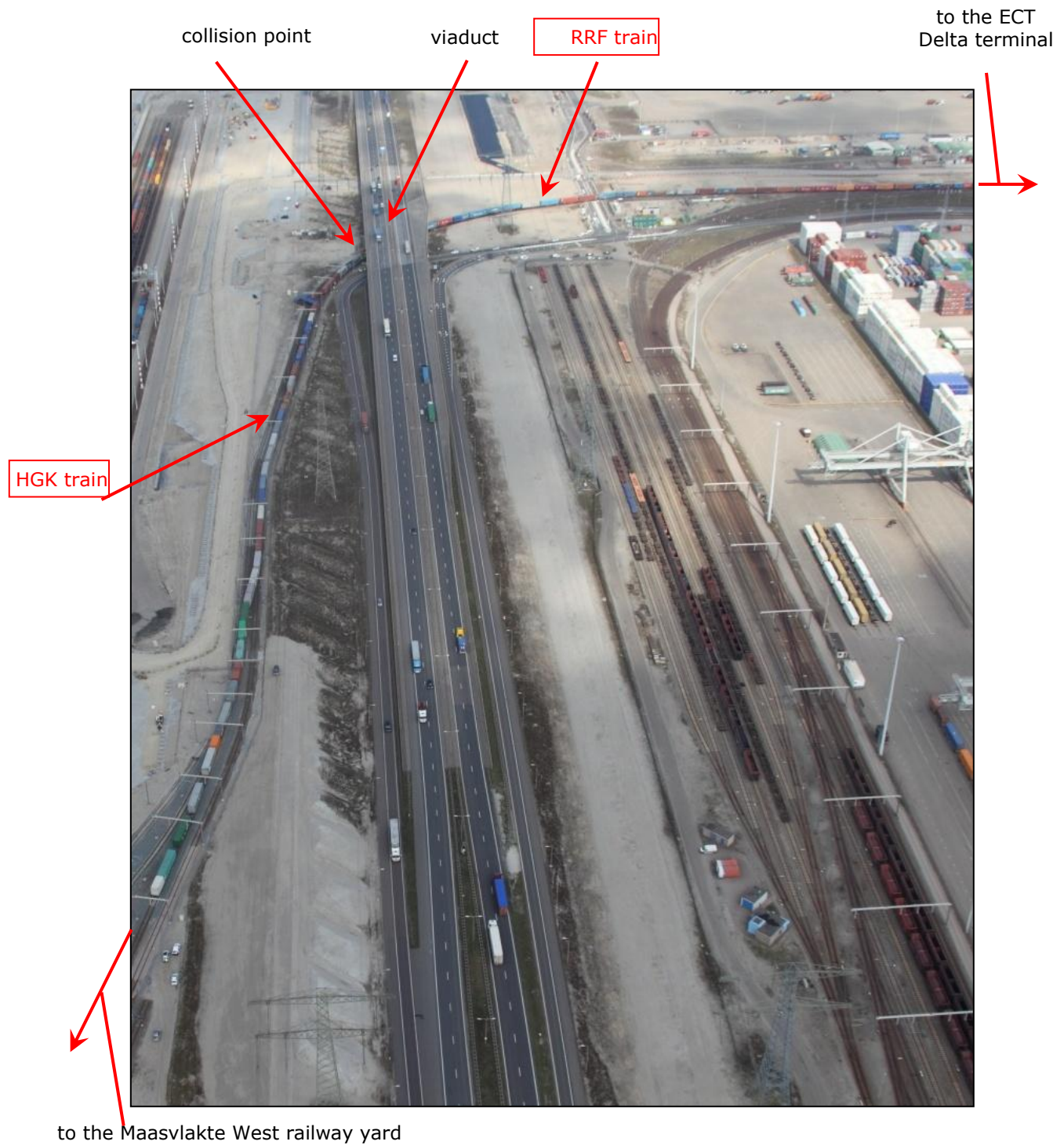
Figure 2: This photo shows the course of the railway tracks and the final positions of both trains.
