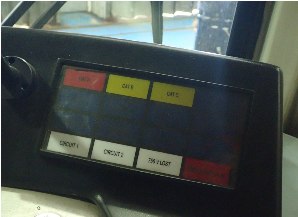
Figure 13: The cab annunciator panel
