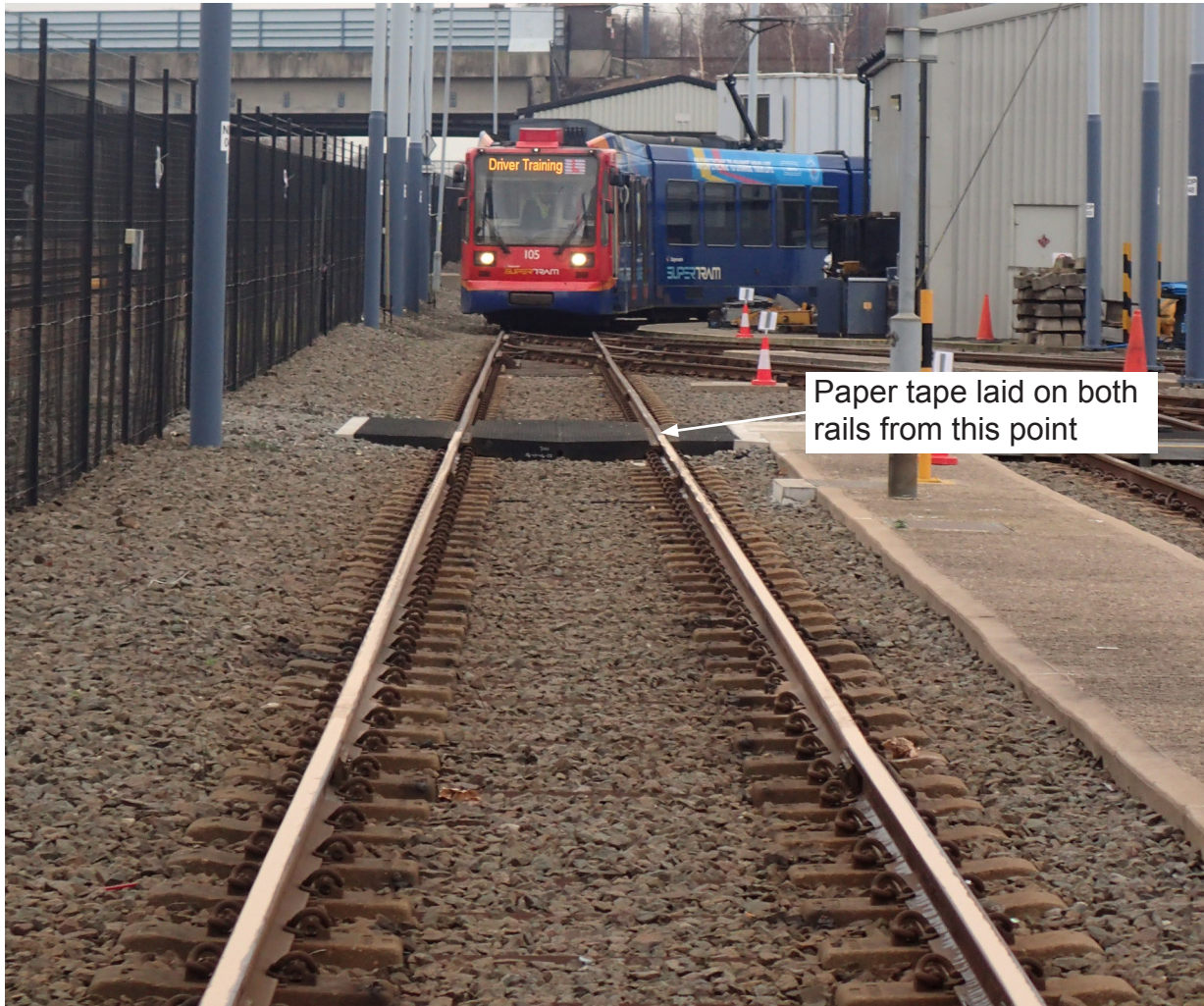
Figure 12: Testing in simulated low adhesion conditions at Nunnery Depot . The tram is moving towards the viewer. Paper tape has been applied to the railhead from the crossing onwards
