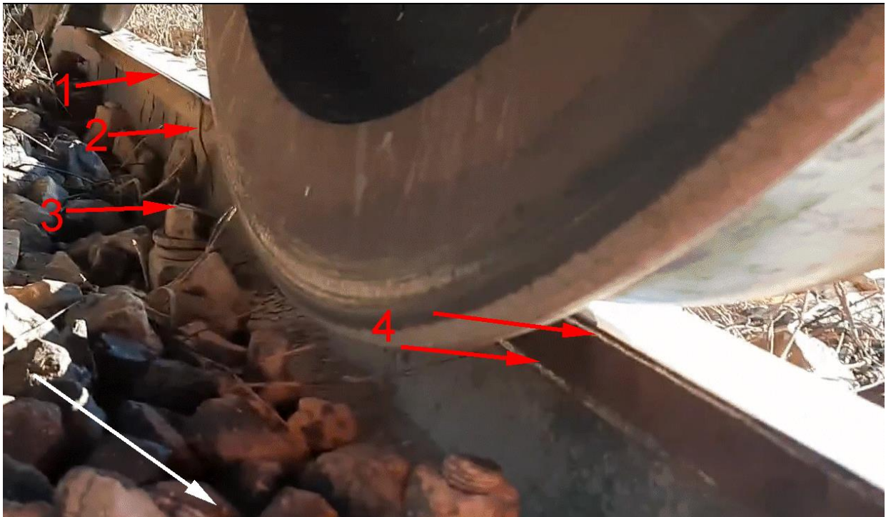
Figure 4.2.1.14: Trace of the first fall of the wheel into the track
