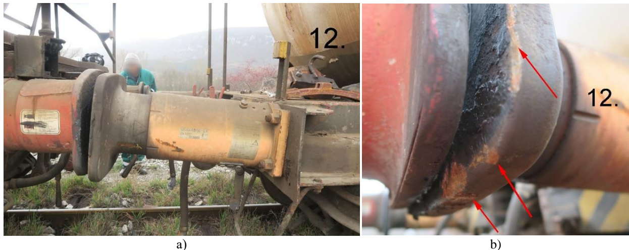
Figure 4.2.1.10: Bent buffer and traces on the buffer plate of the twelfth wagon
