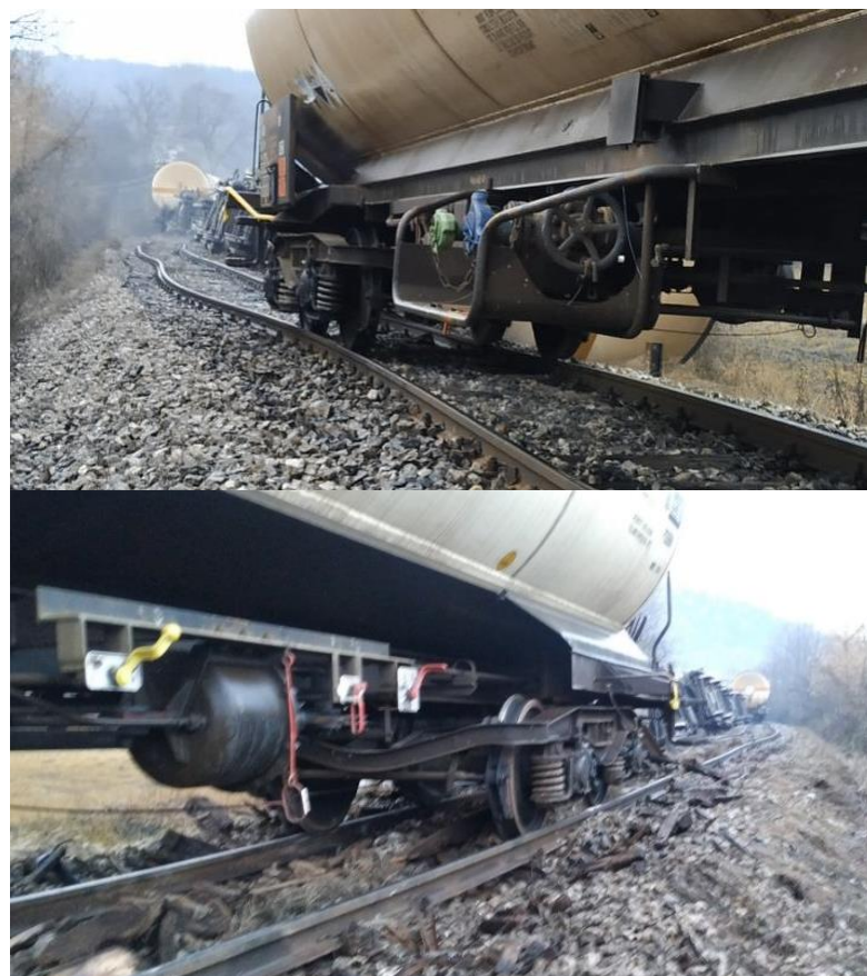
Figure 3.4.4.2: Appearance of the derailed ninth (up) and fourteenth wagon (down) (source: "IŽS" a.d.)
