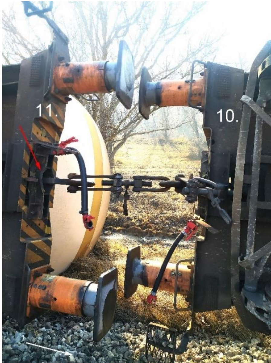
Figure 4.2.1.4: Joint position of the overturned tenth and eleventh wagon
