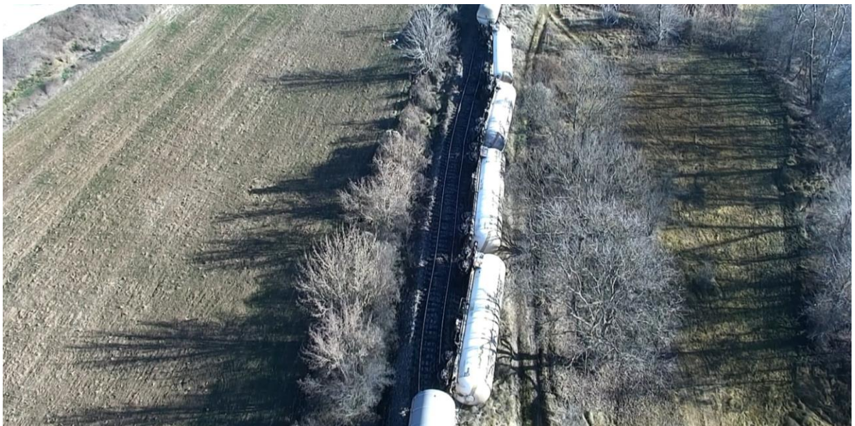
Figure 2.1.2.2: The appearance of the point of overturning of the wagon-tanks (source: MUP, Sector for Emergency Situations)
