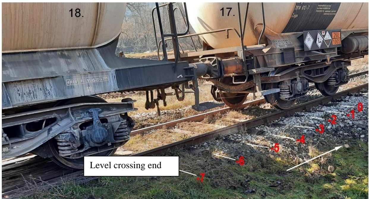
Figure 4.2.1.16: Point of the falling of the wheel into the track (zero sleeper)
