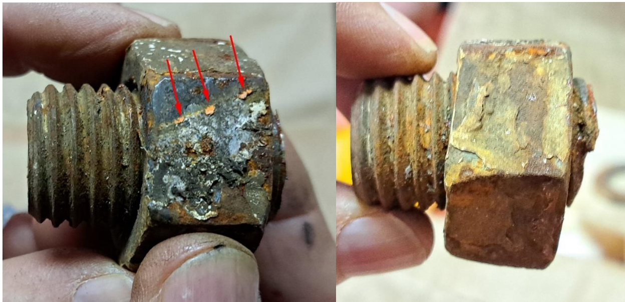
Figure 4.2.1.11: The appearance of the found severed screws
