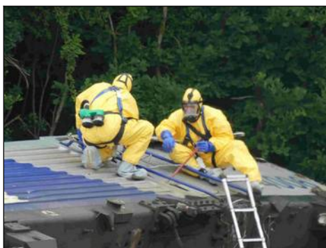
Opening of the locomotive access door and fixing points for the short-circuiting bar
