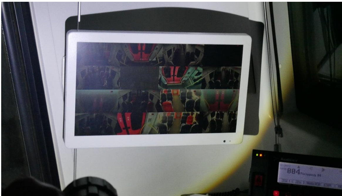
Photo 8 - Driver's cab equipped with CCTV viewing (PKBWK's own material).
