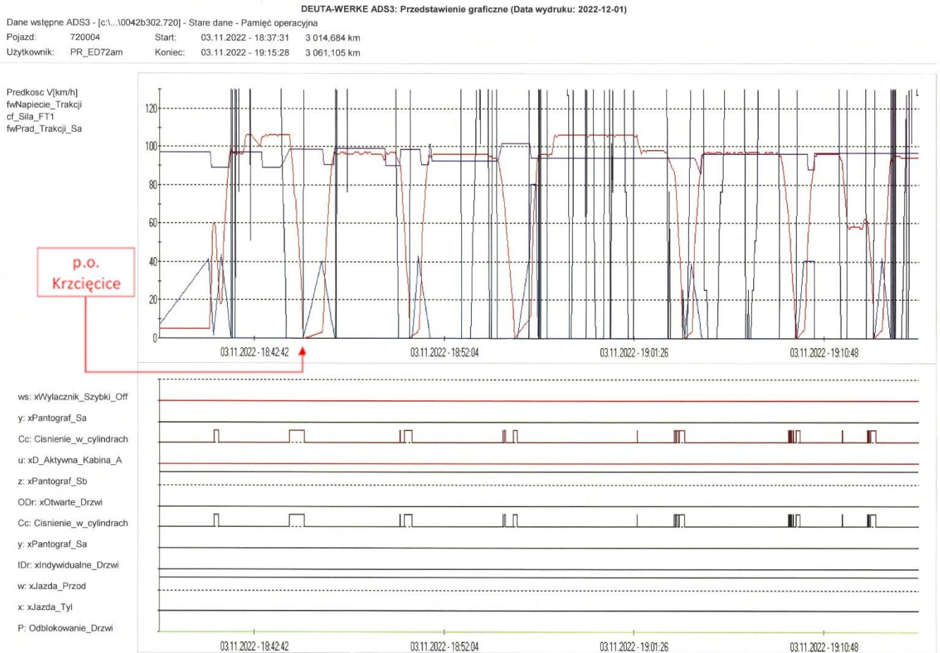
Figure 3 - Graph of driving parameters of the ED72Aa-004 locomotive as a function of time
