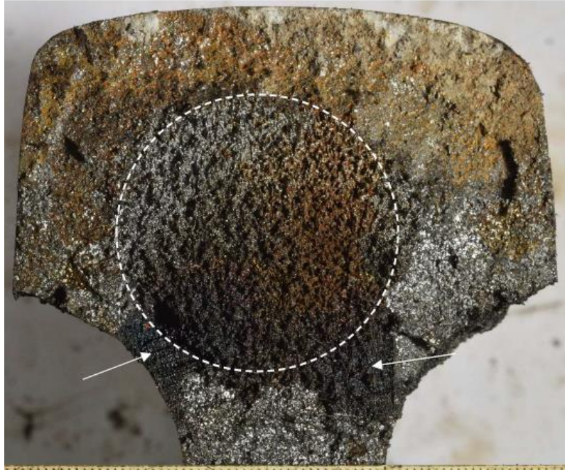
Figure 12 – Fracture face in the head
