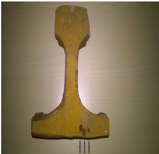
Figure 13 – Rail foot defects
