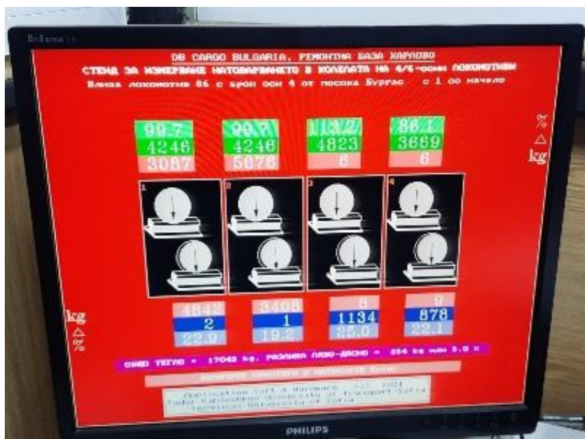
Fig. 2.7. Results from the measurement of the static loading of the wheels of № 21802475039-8 of RBCO Karlovo on 09.05.2024
