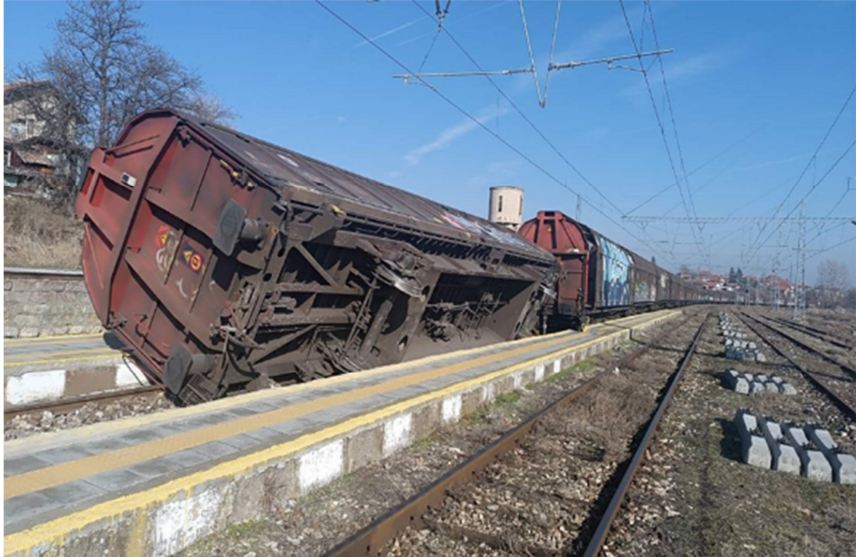
Fig. 2.1. Derailed two last wagons of IDFT № 46660
