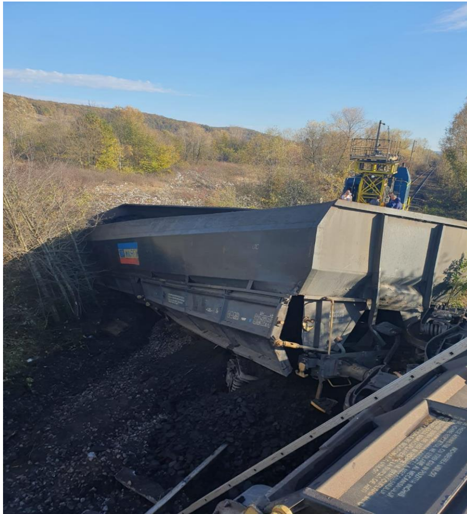
Photo 2: 2nd derailed wagon and 3rd overturned wagon
